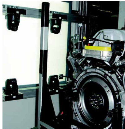
Control of automobile engines with several cameras and special lighting
